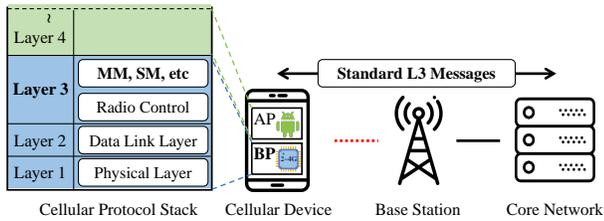
**Fig. 1:** Overall cellular network architecture
