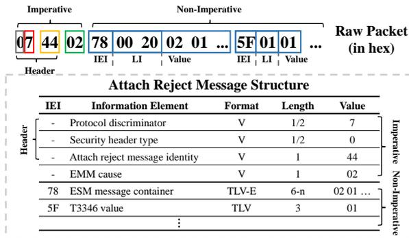
Fig. 2: EMM Attach Reject message structure
