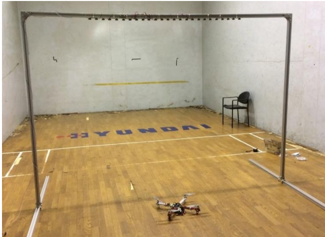
Simple sonic wall (3m-by-2m, 25 speakers)
