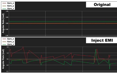
Fig. 15: IMU data from the Pixhawk4 board when a 1.44 V voltage is added to the benign clock signal.
